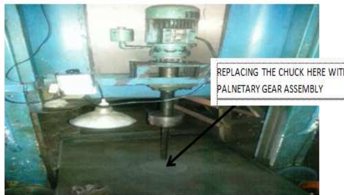
Figure 8: Actual View1 of Machine Where Planetary Gear Assembly is to be Used
